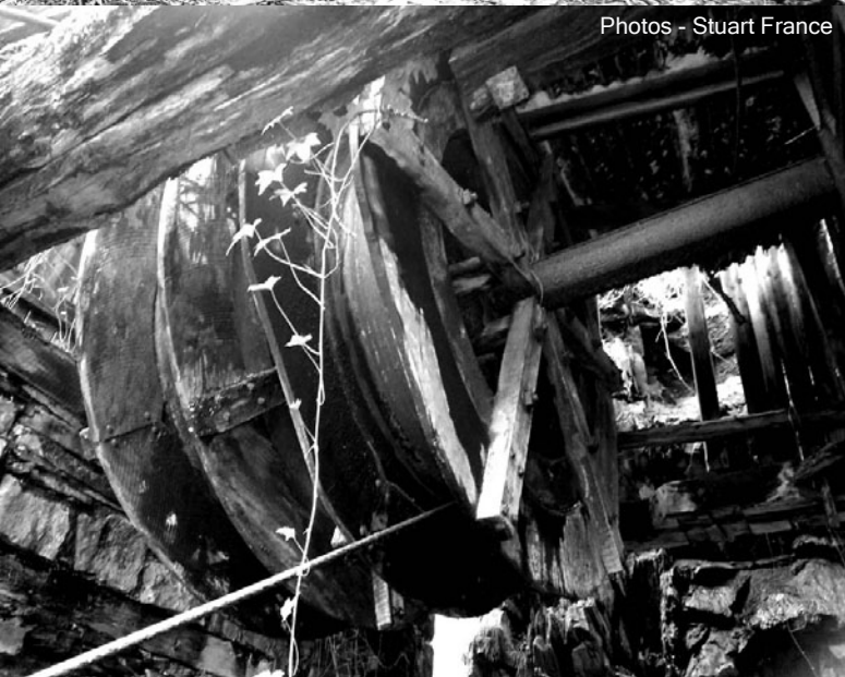
Winding gear at top of new incline
