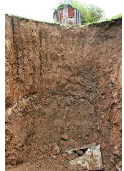
The loess overburden at Vurley 7m deep with angular rock layer
